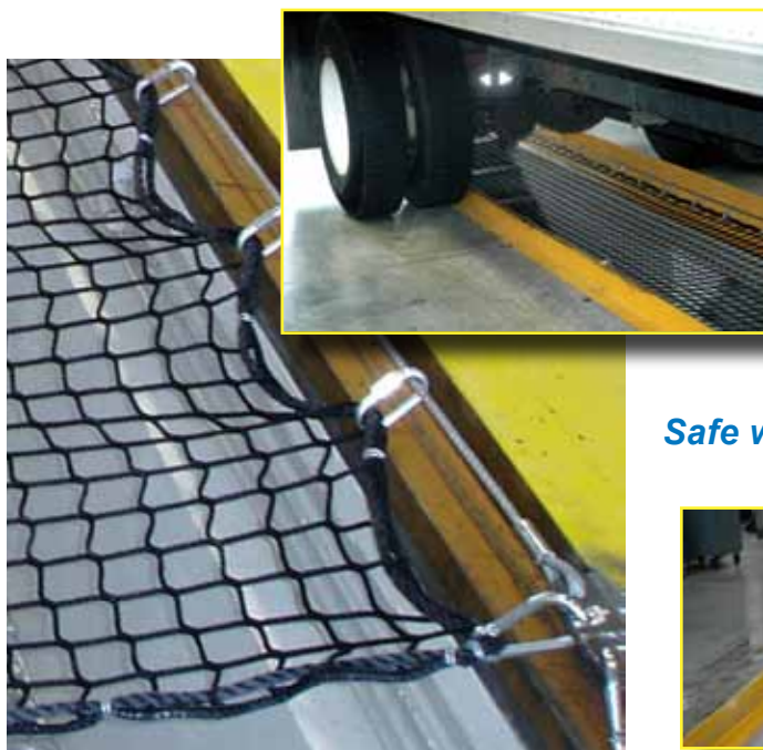
N-820H Polypropylene Knotless Netting 2-1/2 inch square mesh opening, 6000 lb load test.
